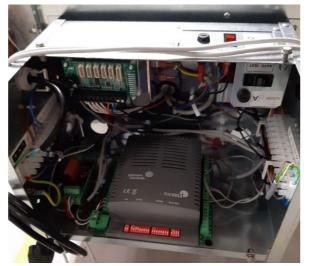
Check for blown fuses. If a fuse is blown check the circuits and components it protects thoroughly before re energising. Any blown fuse must be replaced with an equivalent fuse of the same specification, size and rating.
