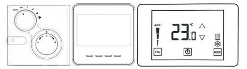
The RCM should be fixed to a wall near to the product within the space that the unit is heating/cooling, away from any cold draughts or radiative heat sources. Wiring to the product should be done with twisted cable with a length of less than 25m.
